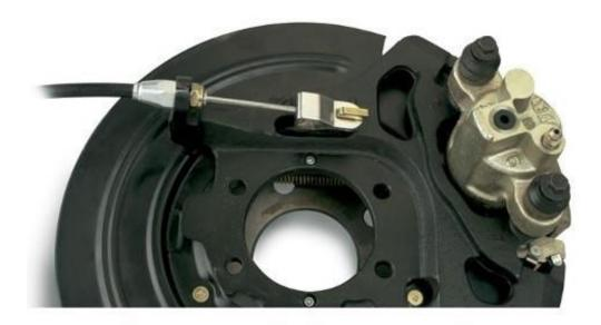
Install the clevises onto the inner wires by sliding the end of the inner wire without the ball end on it through the 1/8" hole from inside the U-shaped part of the clevis. Pull the inner wire through the clevis until the brake cable ball on the end of the inner wire stops inside the clevis. The slotted end of the lever can be installed over the lever at this time.
