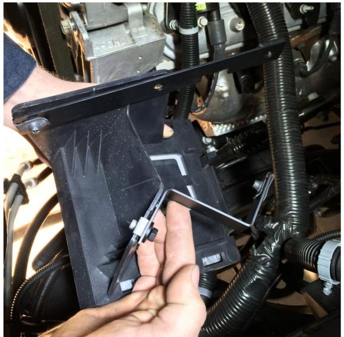
Remove the bolt holding the ECM bracket and loosely install the provided Z bracket and flat strap as shown using the supplied 6mm bolts.
