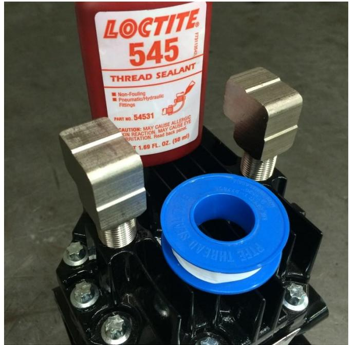
**Standard compressors:** Two 3/8 NPT head fittings are provided with the kit for direct connection to the intake filter and leader hose. Use a thread sealant such as Loctite 545 or Teflon tape to seal the connections to the filter and leader hose. Do not use sealant on the O-ring compressor threads. **SLM compressors:** Thread the provided 90-degree fittings into the head of the compressor using the provided nipples with Loctite 545 or Teflon on both sides of the nipples.
