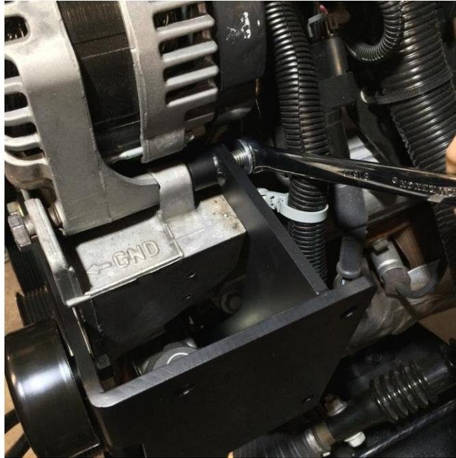
Tighten the fully threaded bolt and then install the M10 nut to sandwich the bracket. The partially threaded M10x130mm bolt should be tightened at this time along with the nut at the back of the power steering pump.
