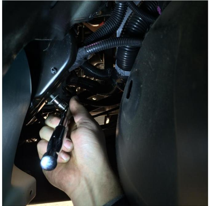
Line up the new strap and Z bracket in place over the existing battery tray holes and reinstall the ECM bracket bolt back into the bottom as shown.
