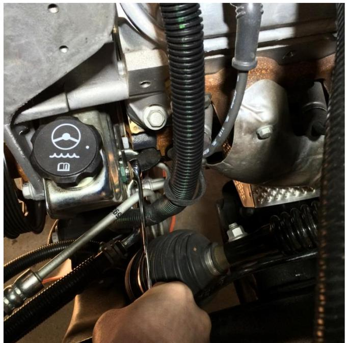
Remove the alternator bolt and accessory bracket bolts as shown. These will no longer be used. Remove the nut at the back of the power steering pump and retain. **NOTE:** Some models have a battery cable bracket attached in the 2 threaded holes shown in **Image 10**. This bracket can be angled by hand to sit behind the new compressor bracket.
