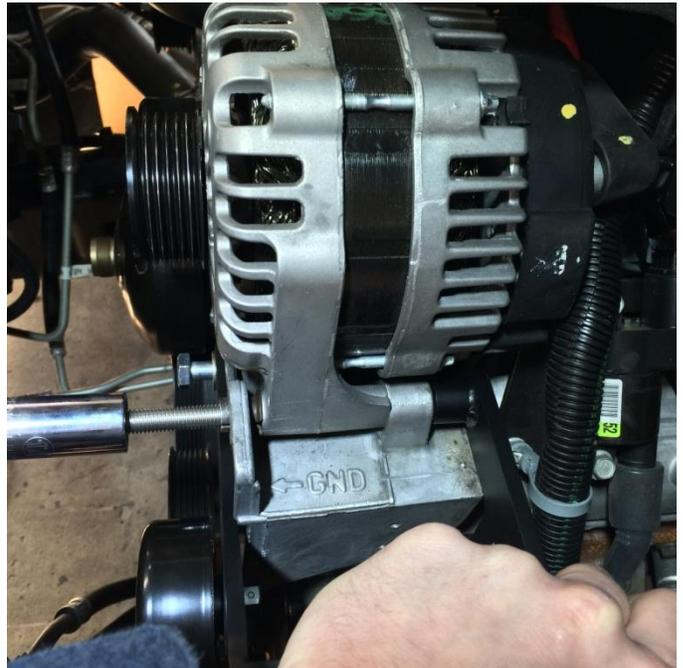
Start the threads of the partially threaded M10x130mm bolt and washer through the bracket. Install the fully threaded M10x130mm through the alternator and the bracket. It may be necessary to align the bracket with the bolt.
