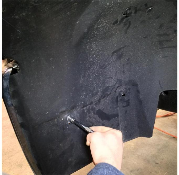
Installation of this system requires shifting the ECU towards the radiator support with the supplied hardware. If your application no longer has the ECU in the stock arrangement, then skip to **Step 7**. Otherwise, remove the battery (most 99-06 models) to access the tray beneath, then remove tray bolts and the tray itself. In the fenderwell, remove the bolts and the associated pushpins that will allow the front of the inner fender to be pulled back for temporary access.
