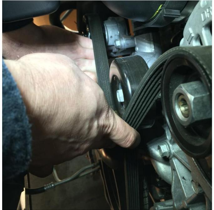
Use a wrench to rotate the tensioner pulley in a clockwise direction until the belt is loose enough to slip off.
