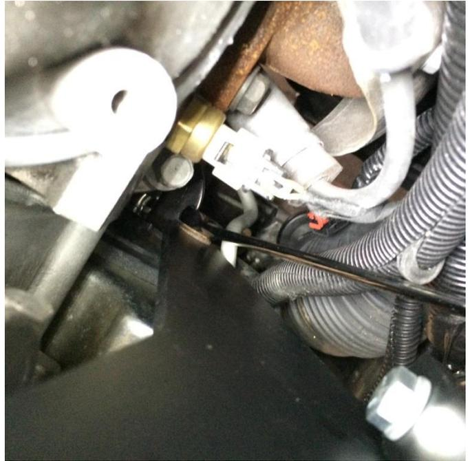
Use a medium strength thread locker (such as Loctite 243) on the nut and reinstall over the new compressor bracket. Start the threads but do not tighten at this time.
