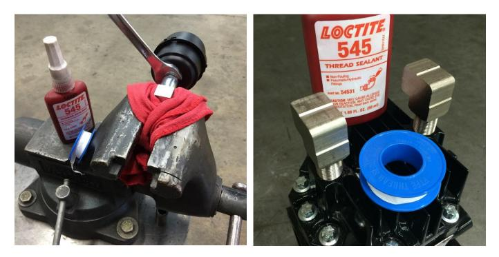
**Standard compressors:** Two 3/8 NPT head fittings are provided with the kit for direct connection to the intake filter and leader hose. Use a thread sealant such as Loctite 545 or Teflon tape to seal the connections to the filter and leader hose. Do not use sealant on the O-ring compressor threads. **SLM compressors:** Thread the provided 90-degree fittings into the head of the compressor using the provided nipples with Loctite 545 or Teflon on both sides of the nipples.
