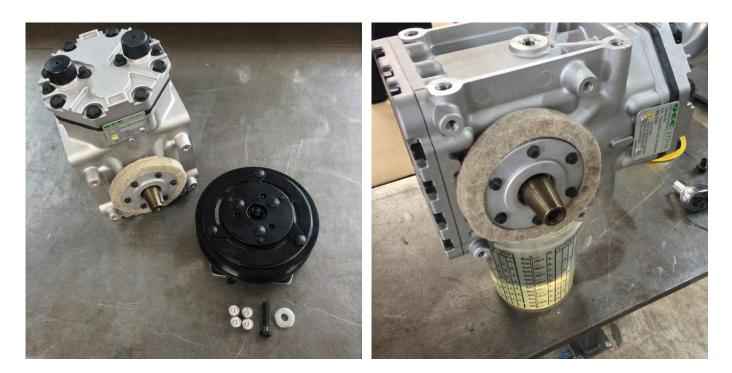
**Standard and SLM compressors:** Verify the new compressor has the half-moon shaped woodruff key installed in the crankshaft. **Standard Compressors only:** The compressors are shipped pre-filled with AC refrigerant oil, but it is recommended to run 12oz of SAE 30 non-detergent engine oil. Remove the bolts from each side of the compressor fill ports and drain the oil.
