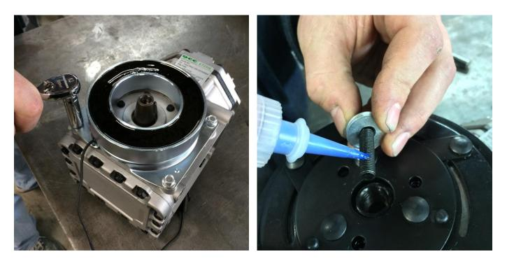
Install and tighten the 4 screws that attach the clutch. You can choose if you want the clutch wire oriented to the top or bottom. Install the 5/16 clutch retainer bolt and torque to **20-25ft lbs**. Never hammer the center bolt onto the snout. Let the screw pull it up until it seats.
