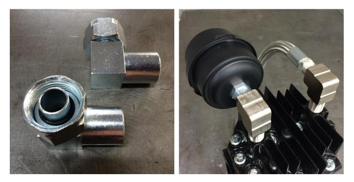
**Standard compressors:** Verify the O-rings are present in the bottom of each of the head fittings and install on the compressor. The filter/silencer will go on the port labeled "Suction". **SLM compressors**: Install the filter/silencer into the suction port side, labeled with an "S". Make sure to hold the 90 fitting with a wrench so as not to break the fitting or compressor head while tightening.
