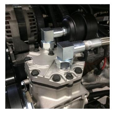
Now is a good time to start the engine and verify there are no problems with the serpentine drive, and that the compressor is not visually out of line.
