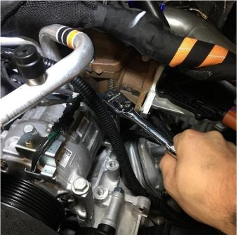
Install the supplied M10x1.5 x 100mm bolt through the idler pulley and machined spacer, then through the factory accessory bracket and secure with the included compression nut. Remove the two factory AC bolts on the driver side.
