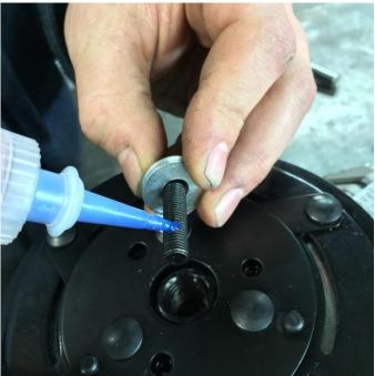
Install and tighten the 4 screws that attach the clutch. You can choose if you want the clutch wiring oriented to the top or bottom. For 8-groove clutches, the white wire is your ground, and the green wire is 12V. Install the clutch retainer bolt and torque to **20-25ft lbs**. (An AC clutch tool such as Mastercool 90499 is best for holding it during installation). Never hammer the clutch onto the snout. Let the screw pull it up until it seats.
