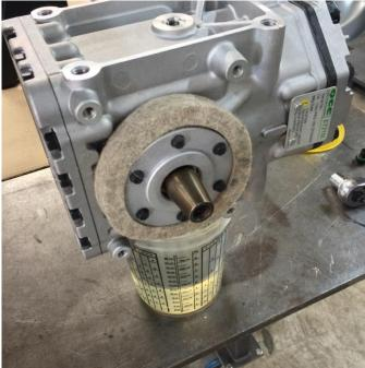
**Standard and SLM compressors:** Verify the new compressor has the half-moon shaped woodruff key installed in the crankshaft. **Standard Compressors only:** The compressors are shipped pre-filled with AC refrigerant oil, but it is recommended to run 12oz of SAE 30 non-detergent engine oil. Remove the bolts from each side of the compressor fill ports and drain the oil.
