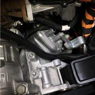
Remove the factory wiring loom from the front of the cast mounting ear and reinstall it into the rear of the same location as shown. Remove the factory belt.
