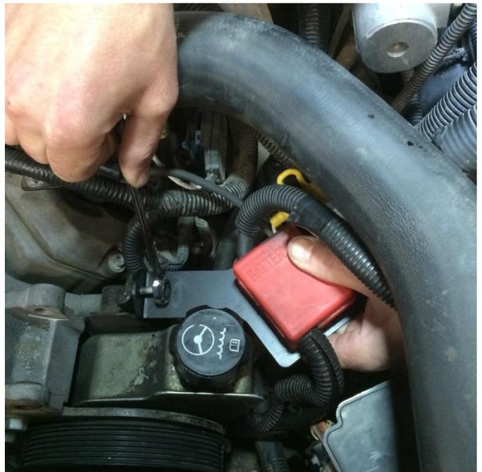
Route the positive battery cable lead underneath the upper radiator hose as shown and then reconnect to the battery and fusebox. The fusebox cover, lid, and fender brace can be reinstalled. The junction box will snap into the new supplied bracket and bolt on with the original bolt.
