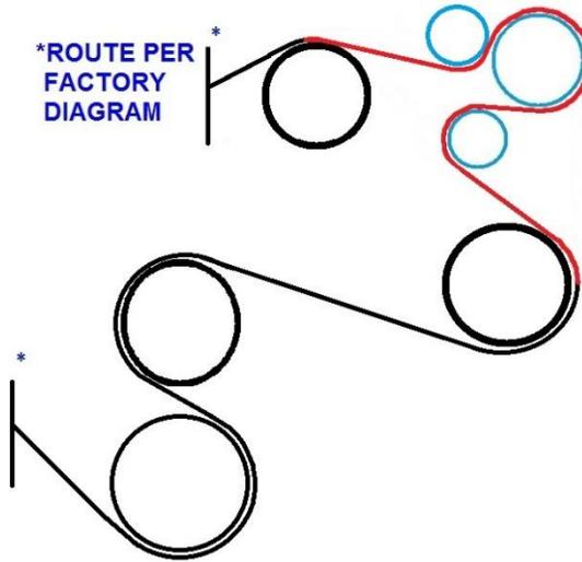
**Alternate Diagram** – Can be used if the primary routing is in between available belt sizes. The top idler pulley would be bypassed.
