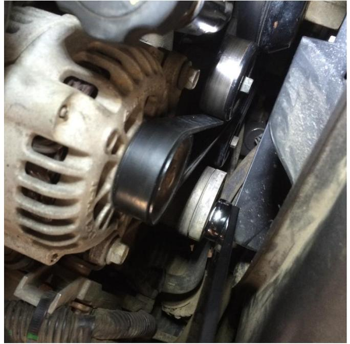
The second idler pulley can now be bolted on using the supplied 3/8 bolt, washers, and locknut.
