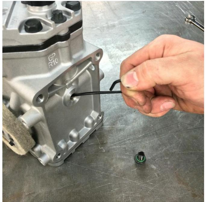
**Standard compressors:** Put one bolt back in and fill with new oil (SAE 30 non-detergent) through the opposite port. It is recommended to use **Valvoline non-detergent SAE 30 (PN 822382)**.
