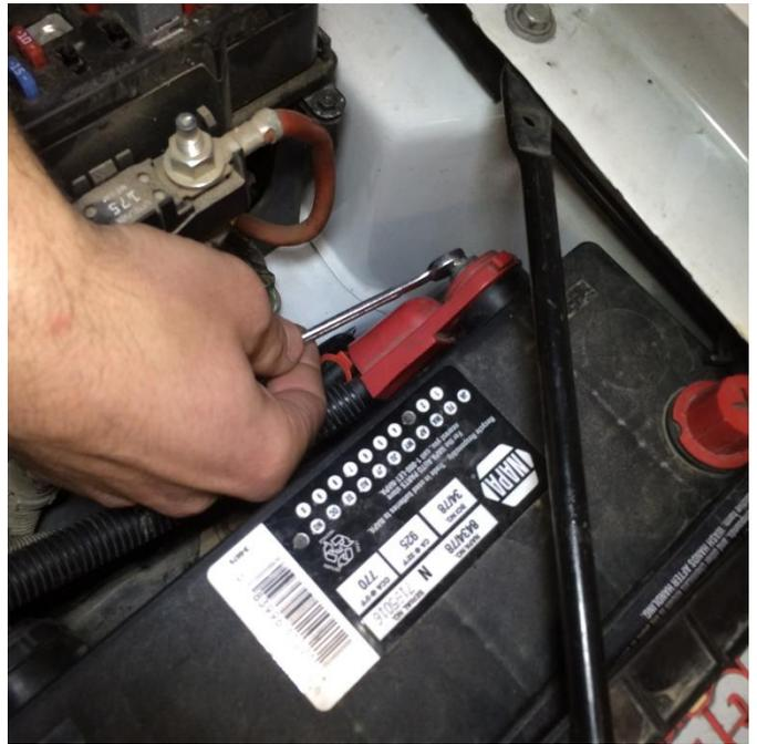
Disconnect the negative battery terminals on BOTH batteries (not shown), then remove the fusebox power wire and the positive terminal on the battery as shown.
