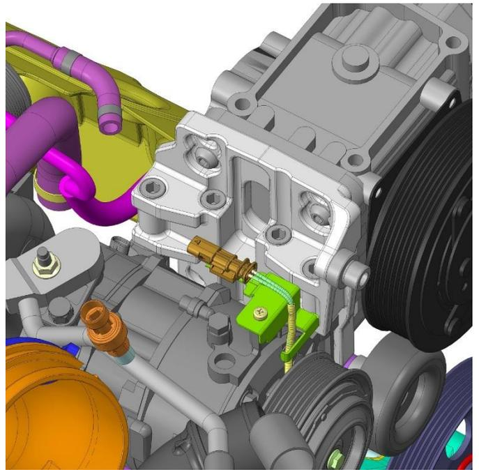
Bolt the compressor to the bracket using **(4) 3/8 x 1.5 bolts** and medium strength threadlocker into the **BOTTOM** set of holes. You will visually center the compressor front to rear in the slots. Its position can be adjusted later if fine-tuned belt alignment is required. The compressor can now be bolted onto the engine using **(4) M10x130mm bolts** with threadlocker.
