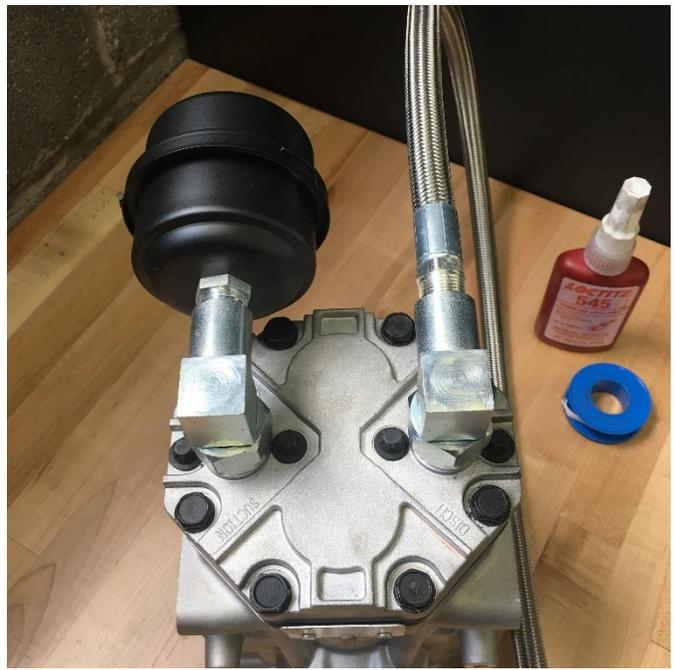
**Standard compressors:** Two 3/8 NPT head fittings are provided with the kit for direct connection to the intake filter and leader hose. Use a thread sealant such as Loctite 545 or Teflon tape to seal the connections to the filter and leader hose. Do not use sealant on the O-ring compressor threads. Verify the O-rings are present in the bottom of each of the head fittings and install on the compressor. The filter/silencer will go on the port labeled "Suction".
