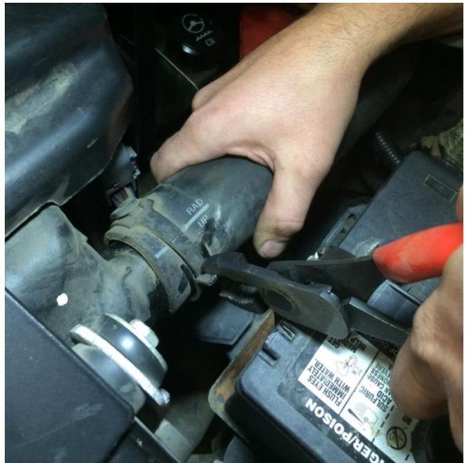
Remove tension from the upper radiator hose clamps. They can be locked into themselves in the open position. Break the seals and slide the hose out approximately 1/4" on each water neck
