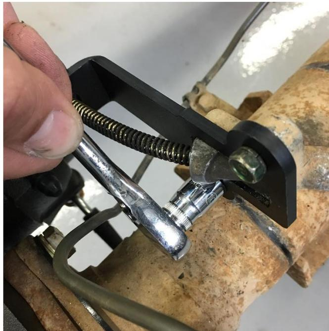
Tighten the 2 bolts into the parking brake cable housing as shown. Special care should be taken to make sure that all parking brake components have adequate clearance to the chassis and moving suspension parts prior to operation of the vehicle. It is suggested to confirm the function of the parking brakes prior to filling and bleeding the hydraulic system
