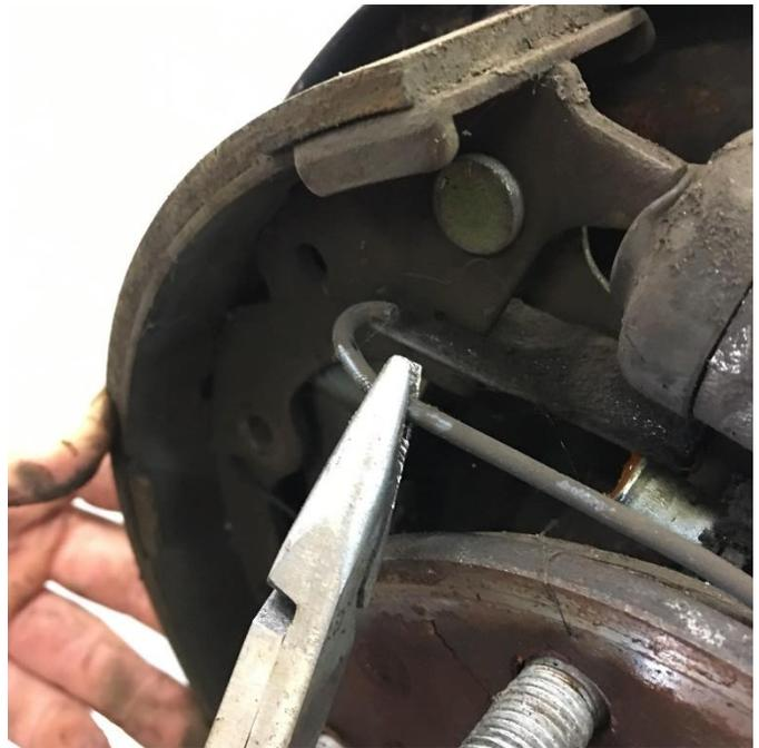
Remove the 2 other retaining springs above and below the axle as shown.
