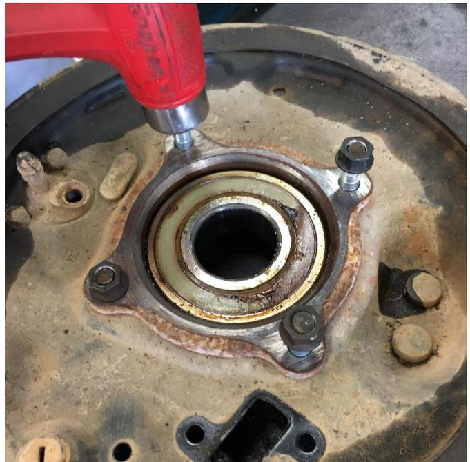
Press the axle out of the backing plate as shown, supporting it as close to the center as possible. Not all presses will have the needed height to perform this operation. Other setups can be used for this, or consult a local automotive shop with experience with Toyota Pickup wheel bearing replacement. After removing the axle, thread the 4 flange nuts back on flush with the tops of the studs, and remove the studs by driving it out with a hammer.
