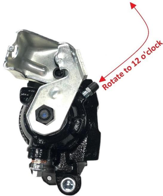
When bleeding this type of parking brake caliper, it is best to temporarily position the caliper so the screw is **vertical to the ground**. If it is not, then it will be necessary to reposition the vehicle, the axle, or the caliper. **If the bleeder screw is not vertical to the ground while bleeding, then you can bleed gallons of fluid through it without eliminating all of the air.**
