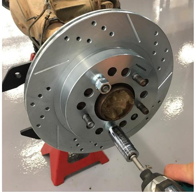
Install the supplied 10-24 screws as shown into locking nuts on the extension bracket side. Do not reinstall the spring yet at this time. Install the rotor using 2 lug nuts to retain it. In the case of drilled/slotted rotors, the direction of rotation shown is for the **passenger side**. **NOTE:** Verify that the rotors are sitting flat against the axle shaft.
