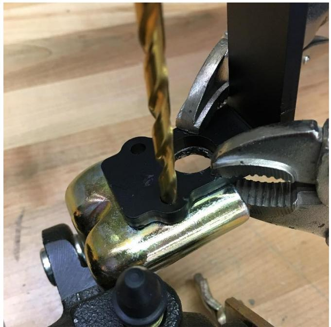
For kits without parking brake calipers, skip to **Step 21**. Remove the spring from the levers and position the cable extension bracket as shown for the passenger side. The hole in the extension bracket will be lined up with the hole in the caliper bracket. Using 2 locking clamps, hold the bracket in position while drilling through the 2 holes using a 3/16 drill bit.
