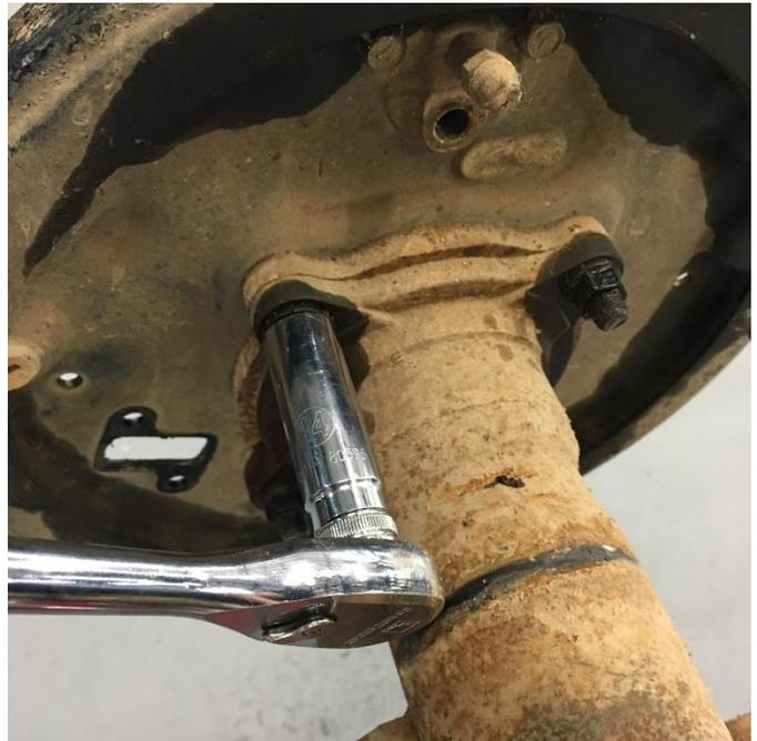
Remove the factory brake line at the back of the drum backing plate. Then remove the 4 bolts securing the axle to the flange. It may be necessary to use a lubricant on these threads.
