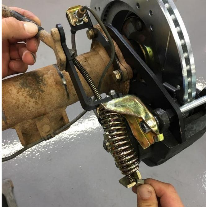
For kits with parking brake calipers, reinstall the factory parking brake cable through the extension bracket and hook to the caliper lever. **NOTE:** Long bed or lifted trucks may require our [Parking Brake Cable Kit](#).
