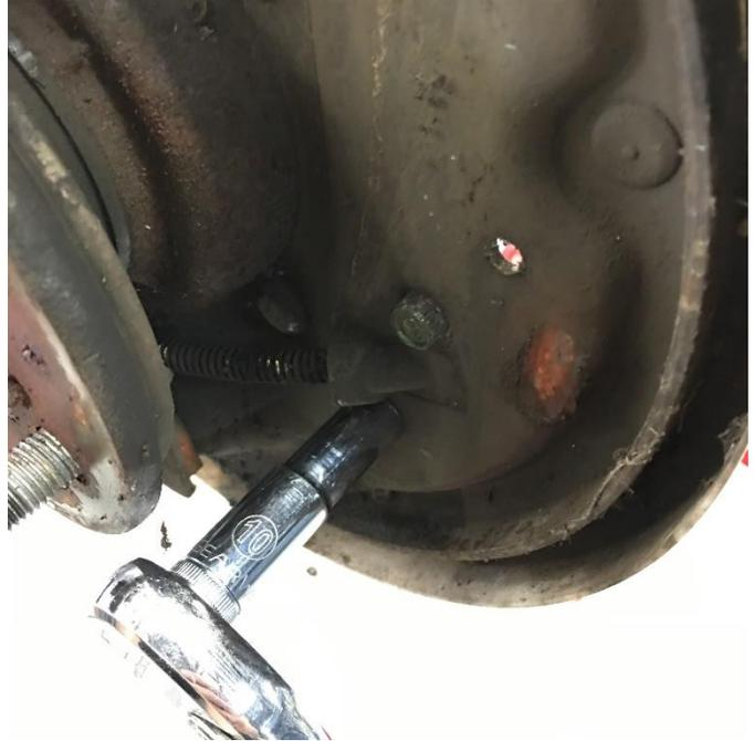
Remove the parking brake cable where it installs into the brake shoe. Then remove the 2 bolts securing it to the drum backing plate. These bolts will need to be kept and reused.
