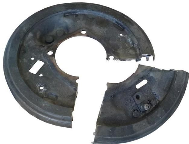
Reinstall the retaining ring, and then install the axle into the housing. **Alternatively to pressing off the bearing:** The user can choose to remove the studs, slip the backing plate down on the axle, then cut a pie shape out as shown using a reciprocating saw or cut-off wheel. When this is done, it is possible to remove the backing plate without removing the bearing from the axle shaft.
