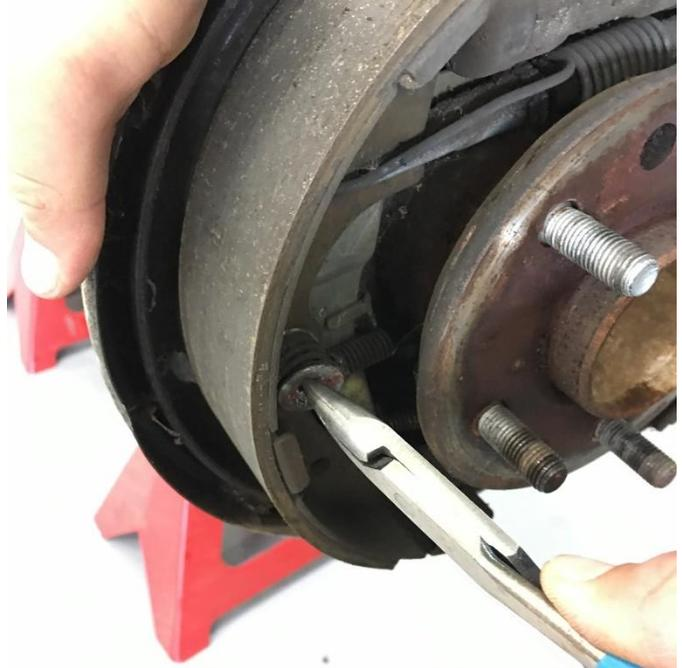
This installation refers to the **passenger side** of the axle. All steps are to be repeated on the driver side. Start by removing the factory drum. It may be necessary use a lubricant around the axle register along with two 5/16-18 bolts threaded into the drum to drive it away from the axle as shown. Once the drum is removed, remove the brake shoe retaining springs (2 places) as shown.
