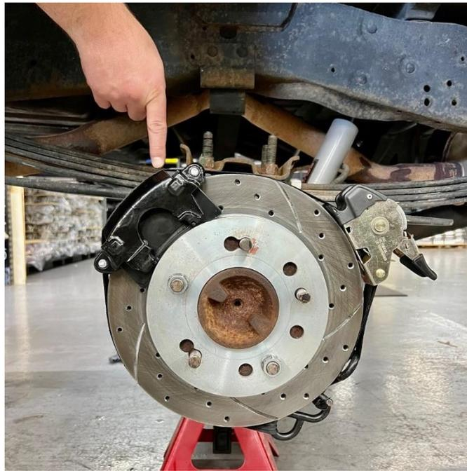
An easy way to accomplish this is to unbolt the main caliper bracket from the axle (leaving the caliper bolted to it) and rotate the caliper around the rotor until the bleeder screw is vertical, then perform the bleeding procedure. Keep the caliper and pads on the rotor during bleeding so that the piston doesn't over-extend outside of its bore.
