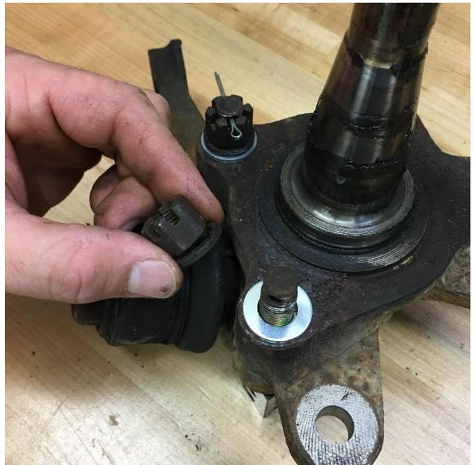
Remove the cotter pins and castle nuts attaching the dust cover to the spindle. The dust cover can be removed and discarded. Reinstall the castle nuts and cotter pins with the new supplied washers to make up for the thickness of the dust cover.
