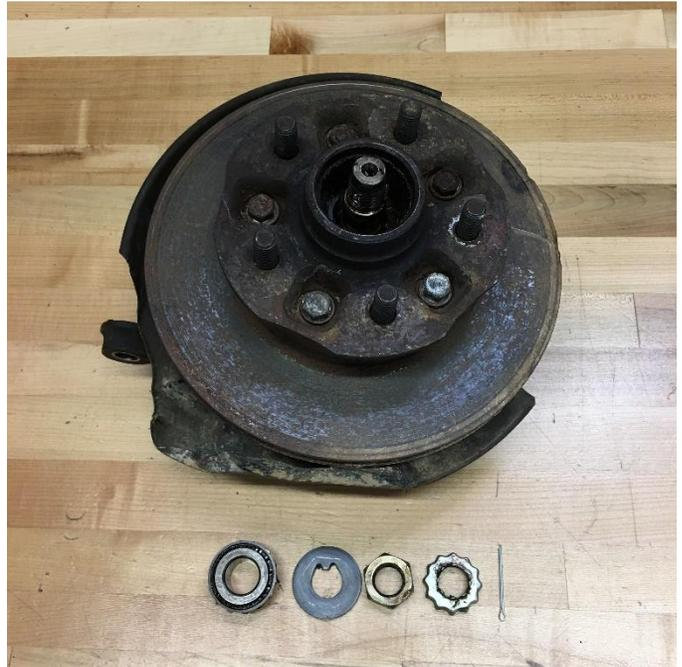
Using a flat head screw driver, remove the dust cap. The cotter pin can then be removed allowing the hub to be removed from the spindle. Do not discard the bearings and hardware, they will be reused.
