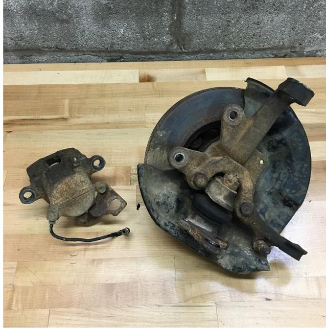
For instruction purposes, the spindle was removed from the vehicle. It is not necessary to remove for the installation of the new brakes. This installation refers to the driver side. All steps are to be repeated on the passenger side in kind. Start by removing the caliper and brake line from the spindle.
