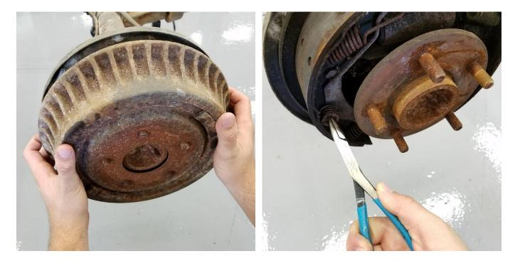
This installation refers to the **passenger side** of the axle. All steps are to be repeated on the driver side. Start by removing the factory drum. It may be necessary use a lubricant around the axle register to do this. Once the drum is removed, remove the brake shoe retaining springs (2 places) as shown.
