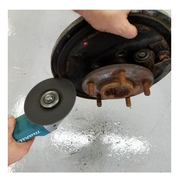
The brackets in this kit are designed to be installed without removing the differential cover. This can be done by use of a cut-off wheel or reciprocating saw to split the drum backing plate into two pieces for removal. If you wish to retain your drum backing plates, the axles can be removed from the housing by draining the fluid, then removing the differential cover, cross pin, and C-clip retainers.
