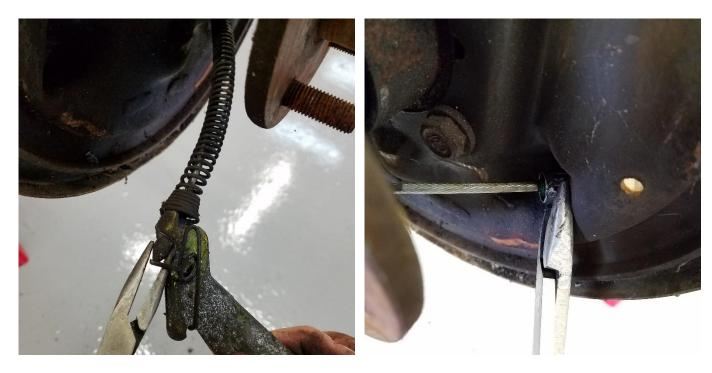
Disconnect the parking brake cable from the brake shoe, then remove and discard the brake shoes and hardware. The cable can then be removed from the backing plate by depressing its perimeter springs.
