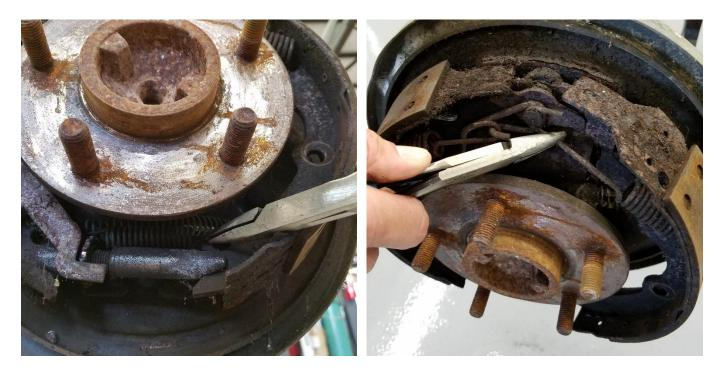
Remove the additional retaining springs from the shoes allowing them to be removed from the backing plate.
