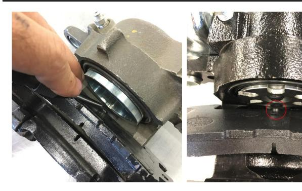
**Kits with non-parking brake calipers** should be checked to confirm the machined pad spacers are present and make sure the notch in the pad spacer lines up with the corresponding boss on the brake pad. **Kits with parking brake calipers** do not use a machined pad spacer and should be checked to confirm the pad is seated flat against the piston face, with the boss of the brake pad lining up with the notch in the piston face.
