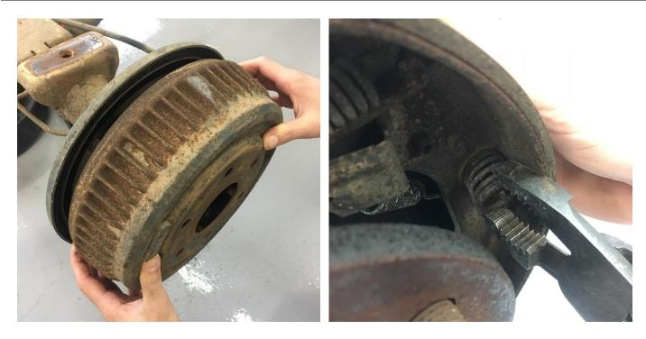
This installation refers to the **passenger side** of the axle. All steps are to be repeated on the driver side. Start by removing the factory drum. It may be necessary use a lubricant around the axle register to do this. Once the drum is removed, remove the brake shoe retaining springs (2 places) as shown.
