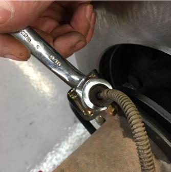
Install the retaining clip as shown, being careful not to bend the hose bracket. The factory brake line can then be repositioned into the top side of the brake line bracket and hose. **Use caution as to not kink the hardline during repositioning.** Next, tighten the brake line nut into your hose. It is best to use a wrench to support the rubber hose from spinning in the key of the hose bracket. **For kits without parking brake calipers, skip to Additional Information and Recommendations.**
