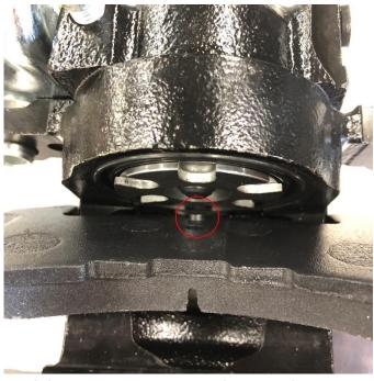
**Normally not required, but in rare cases** the OD of the axle shaft flange may be too large to fit inside of the supplied rotor. If this happens, the solution is to simply remove material from the outside of the axle flange with a sander while rotating the shaft as shown. **Kits with parking brake calipers** should be checked to confirm the pad is seated flat against the piston face, with the boss of the brake pad lining up with the notch in the piston face.
