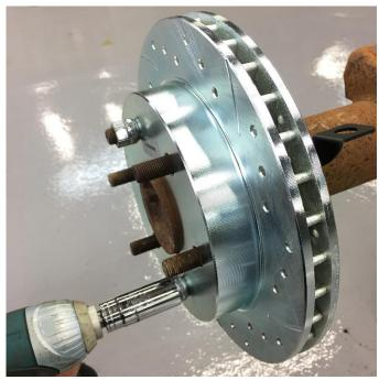
For kits with non-parking brake calipers, bolt on the brackets using the supplied hardware as shown and torque to 20ftlbs. Your caliper should be mounted to the REAR (back) of the axle. For kits with parking brake calipers, temporarily
