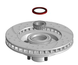
Pack the large inner bearing (A5) with high temperature disc brake bearing grease and install into the back side of the rotor. The inner seal can then be pressed in or lightly tapped in with a hammer by circling the perimeter.
