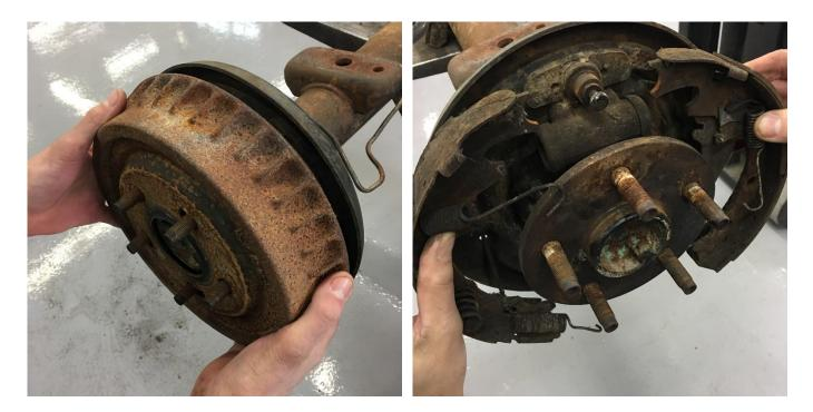
This installation refers to the **driver side** of the axle (unless noted). All steps are to be repeated on the passenger side. Start by removing the factory drum. It may be necessary use a lubricant around the axle register to do this. Once the drum is removed, remove all springs retaining the stock shoes.
