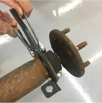
It may be necessary to sand the inboard side of your axle flange to remove any welding slag so that our brackets will bolt up flat to the flange. For kits with non-parking brake calipers, bolt on the brackets using the supplied hardware as shown and torque to 20ft-lbs. Your caliper should be mounted to the REAR (back) of the axle. For kits with parking brake calipers, temporarily leave these bolts loose until the caliper can be bled in the position shown under Parking Brake Caliper Setup.
