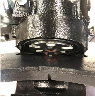
**Kits with non-parking brake calipers** should be checked to confirm the machined pad spacers are present and make sure the notch in the pad spacer lines up with the corresponding boss on the brake pad. **Kits with parking brake calipers** do not use a machined pad spacer and should be checked to confirm the pad is seated flat against the piston face, with the boss of the brake pad lining up with the notch in the piston face.
