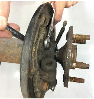
Remove the brake line from the wheel cylinder using a line wrench if possible. The 4 bolts retaining the drum backing plate to the axle can now be removed and discarded.
