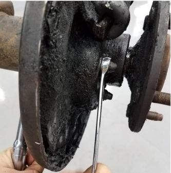
Remove the brake line from the wheel cylinder using a line wrench if possible. The 4 bolts retaining the drum backing plate to the axle can now be removed and discarded.
