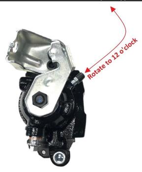
When bleeding this type of parking brake caliper where the bleeder screw is at a 45° angle once installed, we have found that they bleed best when the bleeder screws are at a **vertical 12 o'clock position**. If they are not, then it will be necessary to reposition the vehicle, the axle, or the caliper. **If the bleeder screw is not vertical while bleeding, then you can bleed gallons of fluid through it without eliminating all of the air.**
