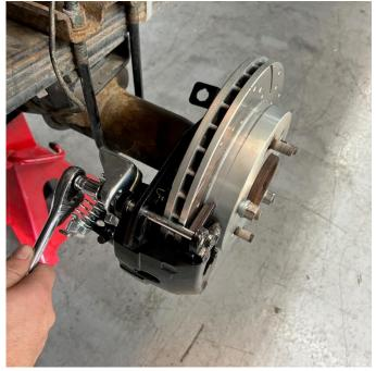
**Kits with parking brake calipers** should be checked to confirm the pad is seated flat against the piston face, with the boss of the brake pad lining up with the notch in the piston face. The calipers can now be installed using medium strength threadlocker (such as Loctite 243) on the threads of the two 7/16-20 caliper bolts. **For parking brake calipers, refer to the instructions below for Parking Brake Caliper Setup**.
