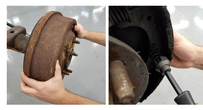
This installation refers to the **passenger side** of the axle. All steps are to be repeated on the driver side. Start by removing the factory drum. It may be necessary use a lubricant around the axle register to do this. Once the drum is removed, remove the brake shoe retaining springs (2 places) as shown.
