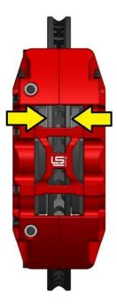
Remove the bridge and bridge bolts and install the pads at this time. Temporarily tighten the lock nuts and view the rotor through the top opening of the caliper. The caliper will need to be centered on the rotor by adding or subtracting the .750x.438x.035 shims between the bracket and the spindle. Always use the same amount of shims on each of the two mounting bolts.
