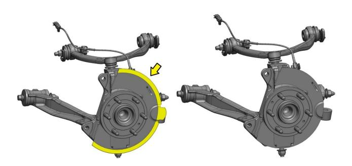
The factory dust shield must be trimmed down to 11.5" in diameter, the area shown in yellow will be removed. A reciprocating saw or metal snips can be used.
