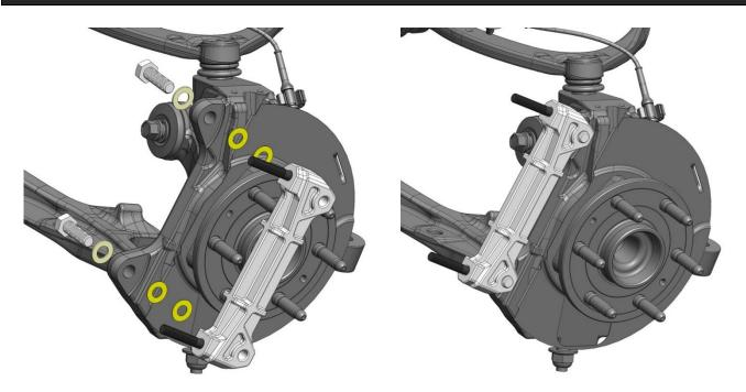
The radial bracket can temporarily be installed at this time using the supplied bolts with flat washers and two .438x.750x.030 shim washers (shown in yellow) between the bracket and spindle. It is not necessary to torque them at this time.
