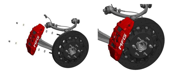
This kit contains distinct right and left-hand calipers that must be mounted in the correct direction. They should be positioned so that the largest pistons are at the rotor exit end of the caliper. Lubricate the caliper mounting studs with lightweight oil. Initially place two .875x.375x.035 shims on each stud of the bracket. Mount the caliper using lock nuts and washers and ensure that it seats on the bracket and does not contact the knuckle.
