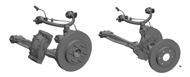
This installation refers to the **passenger side**. All steps are to be repeated on the driver side. For instruction purposes, the knuckle and suspension is shown as being removed, but it is not necessary to remove these components to install new brakes. Start by clamping off the factory brake hose (which is not reused for big brake kits), remove the hose from the caliper, and the caliper with bracket from the knuckle. Next, remove the rotor retaining bolt (if still in place) and rotor.
