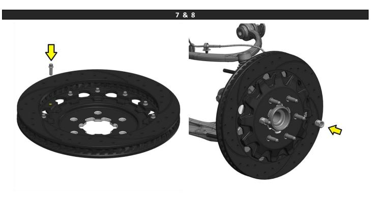
Arrange the rotor and hat in the position shown ensuring the arrow noting rotation direction is correct for its position on the vehicle. Note that the hat should be installed on the flat side of the rotor. Start the first few threads of all 12 of the 5/16-18 x .875 bolts. Using an alternating sequence, apply red Loctite® 271 to the threads, and torque to **25 ft-lbs**. The rotor can be installed on the hub at this time using two lug nuts to hold the hat flat against the hub.
