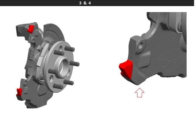
Trim the stock caliper mounting ears first, followed by the tips shown in red. A reciprocating saw, bandsaw, or cut-off wheel can be used. This will be done on both top and bottom ears.
