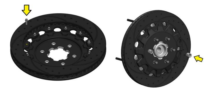
Arrange the rotor and hat in the position shown ensuring the arrow noting rotation direction is correct for its position on the vehicle. Note that the hat should be installed on the flat side of the rotor. Start the first few threads of all 12 of the 5/16-18 x .875 bolts. Using an alternating sequence, apply red Loctite<sup>®</sup> 271 to the threads, and torque to **25 ft-lbs**. The rotor can be installed on the hub at this time using two lug nuts to hold the hat flat against the hub.
