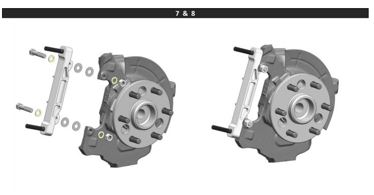
The radial brackets can temporarily be installed at this time using the supplied 7/16 bolts with flat washers and two .438x1.00x.030 shim washers between the bracket and knuckle as shown in step 7. It is not necessary to torque them at this time.
