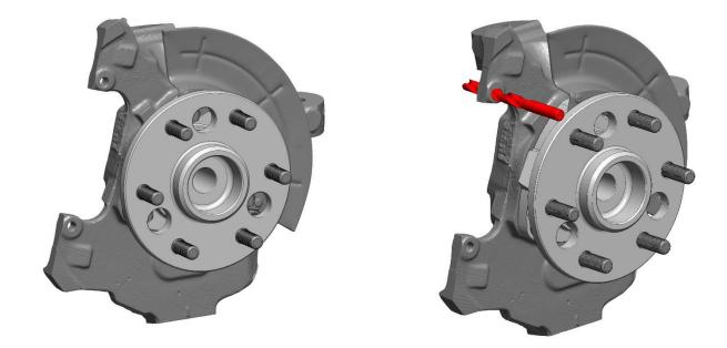
Sand the trimmed surfaces smooth. Any sharp tips left over must be sanded flat to avoid contact with the new caliper radial bracket. Drill the original caliper mounting bolt holes with a 7/16 drill bit (not included). Check the drilled area for burs and sand smooth if necessary.
