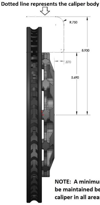
NOTE: A minimum of .125" clearance must be maintained between the wheel and caliper in all areas
