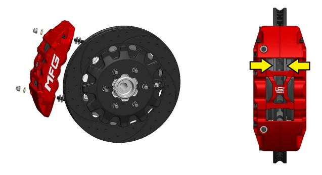
This kit contains distinct right and left-hand calipers that must be mounted in the correct direction. They should be positioned so that the largest pistons are at the rotor exit end of the caliper. Lubricate the caliper mounting studs with lightweight oil. Initially place two .438x.750x.030 shims on each stud of the bracket. Mount the caliper using lock nuts and washers and ensure that it seats on the bracket and does not contact the knuckle.
