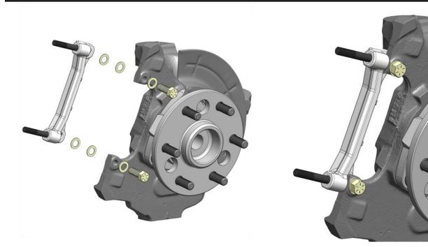
The radial brackets can temporarily be installed at this time using the supplied 7/16 bolts with flat washers and two .750x.438x.035 shim washers between the bracket and knuckle as shown in step 7. It is not necessary to torque them at this time.
