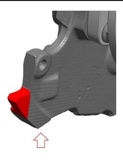
Trim the stock caliper mounting ears first, followed by the tips shown in red. A reciprocating saw, bandsaw, or cut-off wheel can be used. This will be done on both top and bottom ears.
