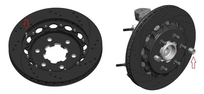
Arrange the rotor and hat in the position shown (to the flat side of the rotor) ensuring the arrow noting rotation direction is correct for its position on the vehicle. Start the first few threads of all 12 of the ½-20 x .75 12-point bolts. Using an alternating sequence, apply red Loctite® 271 to the threads, and torque to **155 in-lbs**. The rotor can be installed on the hub at this time using two lug nuts to hold the hat flat against the hub.
