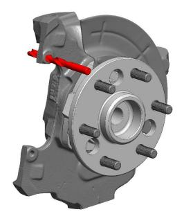
Sand the trimmed surfaces smooth. Any sharp tips left over must be sanded flat to avoid contact with the new caliper radial bracket. Drill the original caliper mounting bolt holes with a 7/16 drill bit (not included). Check the drilled area for burs and sand smooth if necessary.
