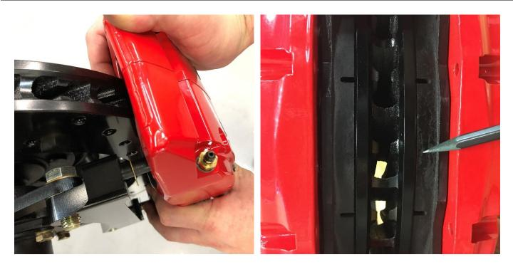
Lubricate the caliper mounting studs with lightweight oil. Initially place one .438x.1.0x.035 shim on each stud of the bracket. Mount the caliper using lock nuts and washers and ensure that it fully seats on the bracket and does not contact the rotor.
