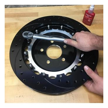
Arrange the rotor and hat in the position shown ensuring the arrow noting rotation direction is correct for its position on the vehicle. Start the first few threads of all 12 of the 5/16-18 x 1" bolts. Using an alternating sequence, apply red Loctite<sup>®</sup> 271 to the threads, and torque to **25 ft-lbs**.
