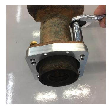
Install the adapter using the hardware provided in the top 2 axle flange holes as shown. The dimples will be mounted **UP** and **OUT** when installed properly. The 10" axle flange adapter is shown in these pics. **If you have the 11" axle flange adapter**, all 4 mounting bolts will start from the outside and go into your axle flange.
