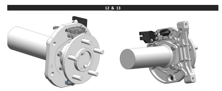
Bolt on the machined backing plate using the supplied hardware, as shown. The calipers should be mounted to the **REAR** of the axle, with the parking brake lever at the top. The radial brackets can temporarily be installed at this time using the supplied M14 bolts and washers, along with two .563x1.125x.035 shim washers between the backing plate and radial bracket.
