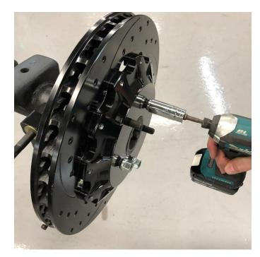
The rotor can be installed on the hub at this time using two lug nuts to hold the hat flat against the hub.
