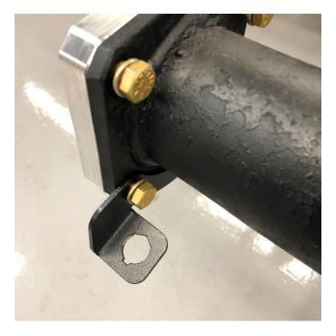
Install the brake line bracket using the hardware provided in the bottom 2 axle flange holes as shown, with the tab towards the **FRONT** of the axle. The 10" axle flange adapter is shown in these pics. **If you have the 11" axle flange adapter**, you will install nuts in this location to retain your brake line bracket.
