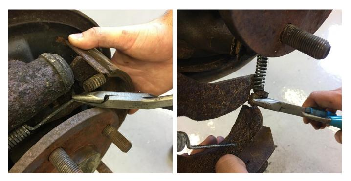
Remove the additional retaining springs from the brake shoes. Disconnect the parking brake cable from the brake shoe, then remove and discard the brake shoes and hardware.
