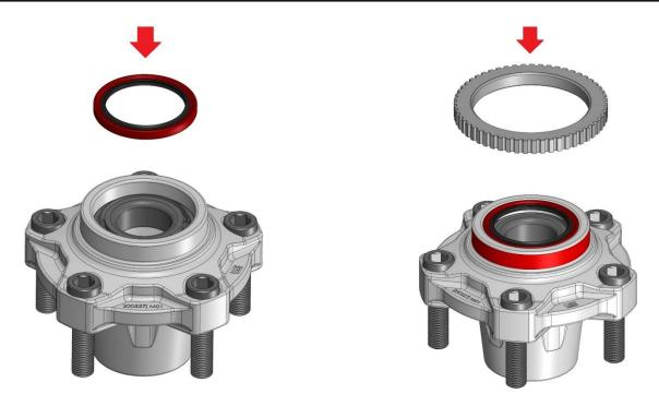
Pack the large inner bearing (A5) with high temperature disc brake bearing grease and install into the back side of the hub. The inner seal can then be pressed in or lightly tapped in with a hammer by circling the perimeter. **If your truck has front wheel ABS**, remove the reluctor ring from the stock rotor and install it onto the hub.
