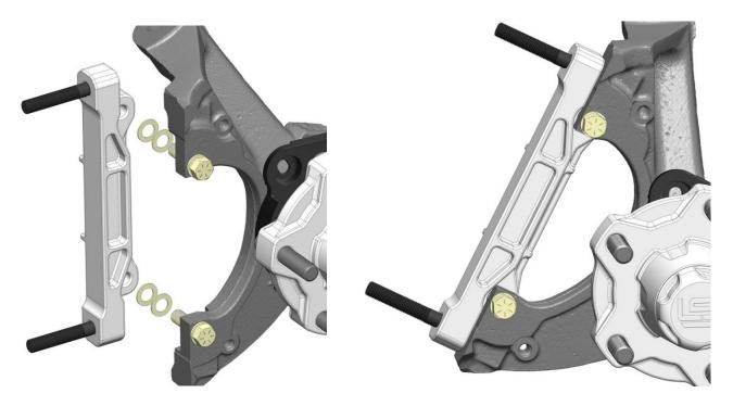
The radial bracket can temporarily be installed at this time using the supplied bolts with flat washers and two .438x1.00x.030 shim washers between the bracket and spindle. It is not necessary to torque them at this time.
