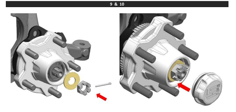
If your truck has front wheel ABS, the ABS sensor will be remounted to the spindle using the bolt hole it previously used on the dust shield. You can now install the hub onto the spindle, then pack the outer bearing (A3) with grease and install under the factory washer, castle nut, and supplied cotter pin. After bending the leg of the cotter pin, install the machined dust cap as shown.
