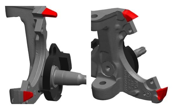
Trim the spindle ears as shown. A reciprocating saw, bandsaw, or cut-off wheel can be used.
