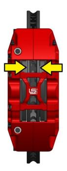
This kit contains distinct right and left-hand calipers that must be mounted in the correct direction. They should be positioned so that the largest pistons are at the rotor exit end of the caliper. Lubricate the caliper mounting studs with lightweight oil. Initially place two .438x.750x.030 shims on each stud of the bracket. Mount the caliper using lock nuts and washers and ensure that it seats on the bracket and does not contact the spindle.
