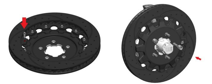
Arrange the rotor and hat in the position shown ensuring the arrow noting rotation direction is correct for its position on the vehicle. Note that the hat should be installed on the flat side of the rotor. Start the first few threads of all 12 of the 5/16-18 x .875 bolts. Using an alternating sequence, apply red Loctite® 271 to the threads, and torque to **25 ft-lbs**. The rotor can be installed on the hub at this time using two lug nuts to hold the hat flat against the hub.
