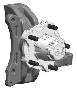
You can now install the hub onto the spindle, then pack the outer bearing (A3) with grease and install under the factory washer, castle nut, and supplied cotter pin. After bending the leg of the cotter pin, install the machined dust cap as shown.
