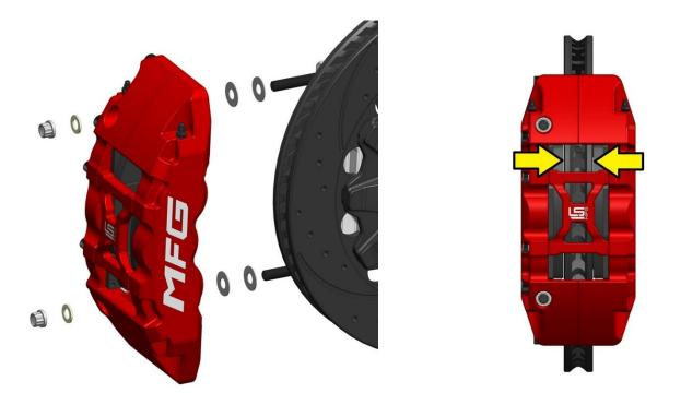
This kit contains distinct right and left-hand calipers that must be mounted in the correct direction. They should be positioned so that the largest pistons are at the rotor exit end of the caliper. Lubricate the caliper mounting studs with lightweight oil. Initially place one .438x1.0x.030 shim on each stud of the bracket. Mount the caliper using lock nuts and washers and ensure that it seats on the bracket and does not contact the spindle.
