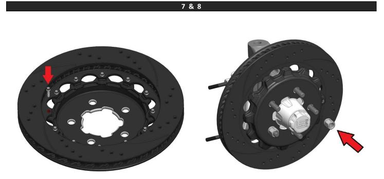
Arrange the rotor and hat in the position shown ensuring the arrow noting rotation direction is correct for its position on the vehicle. Note that the hat should be installed on the flat side of the rotor. Start the first few threads of all 12 of the 5/16-18 x .875 bolts. Using an alternating sequence, apply red Loctite<sup>®</sup> 271 to the threads, and torque to **25 ft-lbs**. The rotor can be installed on the hub at this time using two lug nuts to hold the hat flat against the hub.
