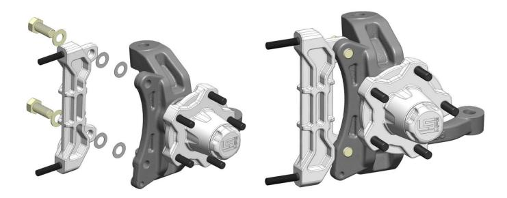
The radial bracket can temporarily be installed at this time using the supplied bolts with flat washers and two .750x.438x.030 shim washers between the bracket and spindle. It is not necessary to torque them at this time.
