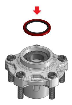
Pack the large inner bearing (A5) with high temperature disc brake bearing grease and install into the back side of the hub. The inner seal can then be pressed in or lightly tapped in with a hammer by circling the perimeter.
