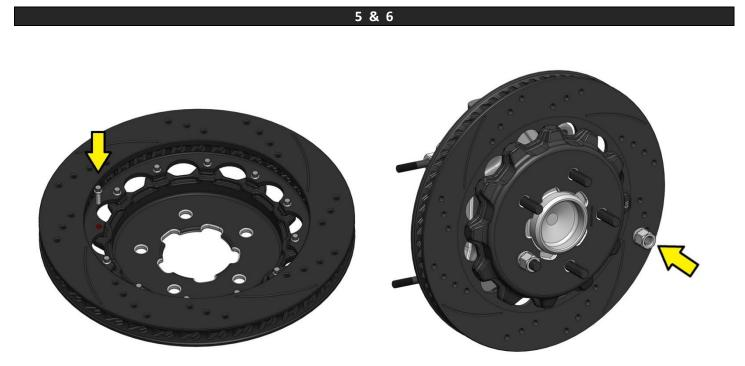
Arrange the rotor and hat in the position shown ensuring the arrow noting rotation direction is correct for its position on the vehicle. Note that the hat should be installed on the flat side of the rotor. Start the first few threads of all 12 of the ¼-20 12-point bolts. Using an alternating sequence, apply red Loctite<sup>®</sup> 271 to the threads, and torque to **155 in-lbs**. The rotor can be installed on the hub at this time using two lug nuts to hold the hat flat against the hub.
