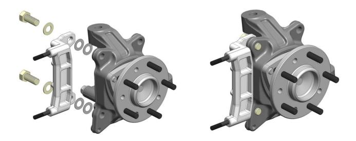
The radial bracket can temporarily be installed at this time using the supplied bolts with flat washers and two .750x.438x.030 shim washers between the bracket and spindle. It is not necessary to torque them at this time.
