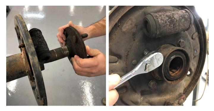
The axles will need to be removed from the housing by draining the fluid, then removing the differential cover, cross pin, and C-clip retainers. The 4 bolts retaining the drum backing plate to the axle can now be removed and discarded.
