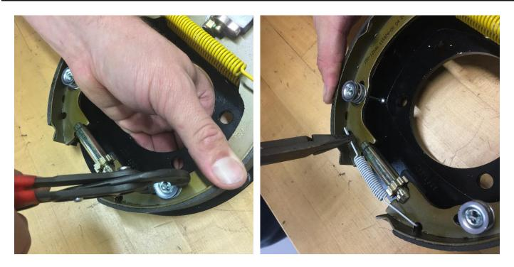
Reinstall the shoe retaining springs as shown, and then finish by reinstalling the bottom spring over the adjuster. At this time, the adjuster should be in the innermost position but not be bottomed out and difficult to adjust through the slotted window after assembly.
