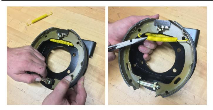
After installing the new bracket, you can now begin reassembly of the brake shoes. Start by installing the inside top retaining spring and assemble the shoes onto the backing plate. Then insert the tensioner and then install the outside top spring.
