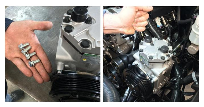
Four 3/8 bolts and lock washers are provided for mounting the compressor to the bracket. They should be tight but be careful not to strip the aluminum compressor body.
