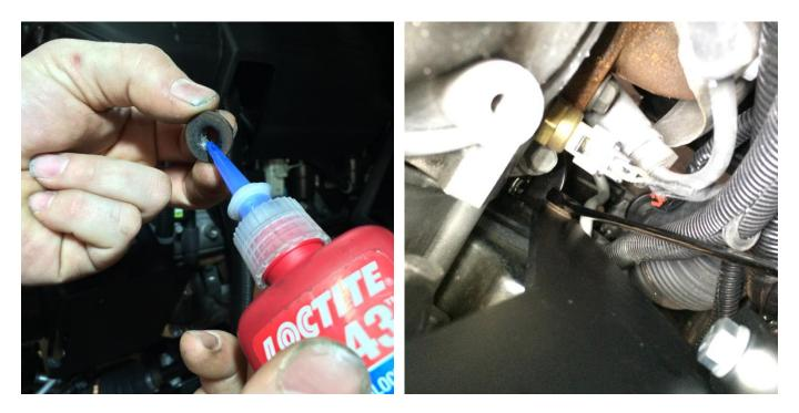
Use a medium strength thread locker (such as Loctite 243) on the nut and reinstall over the new compressor bracket. Start the threads but do not tighten at this time.
