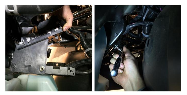
Line up the new strap and Z bracket in place over the existing battery tray holes and reinstall the ECM bracket bolt back into the bottom as shown.
