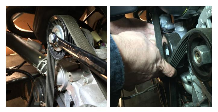
Use a wrench to rotate the tensioner pulley in a clockwise direction until the belt is loose enough to slip off.
