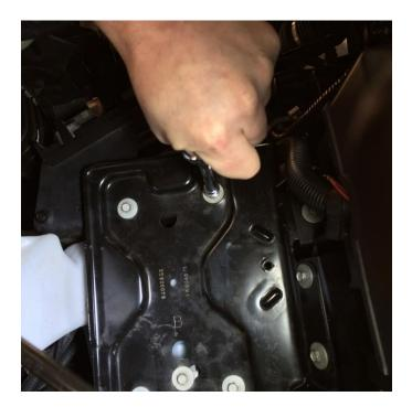
Tighten the tray bolts back through their original holes. The ECM has now been shifted to accommodate the engine driven compressor.
