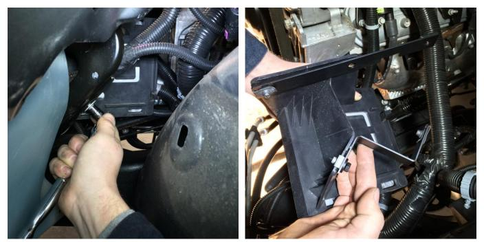
Remove the bolt holding the ECM bracket and loosely install the provided Z bracket and flat strap as shown using the supplied 6mm bolts.
