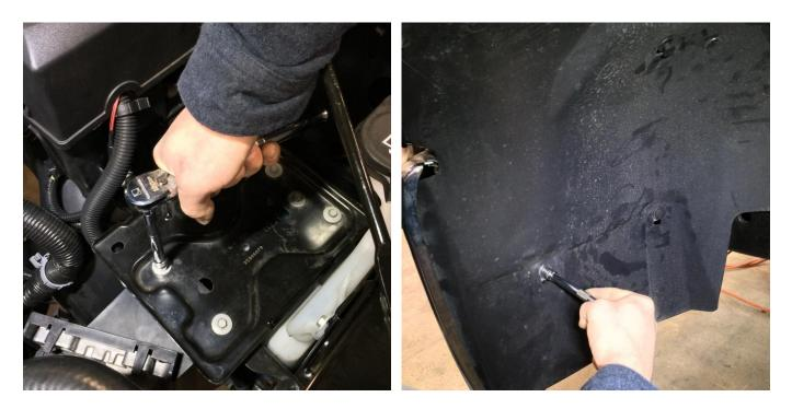
Installation of this system requires shifting the ECU towards the radiator support with the supplied hardware. If your application no longer has the ECU in the stock arrangement, then skip to **Step 7**. Otherwise, remove the battery (most 99-06 models) to access the tray beneath, then remove tray bolts and the tray itself. In the fenderwell, remove the bolts and the associated pushpins that will allow the front of the inner fender to be pulled back for temporary access.
