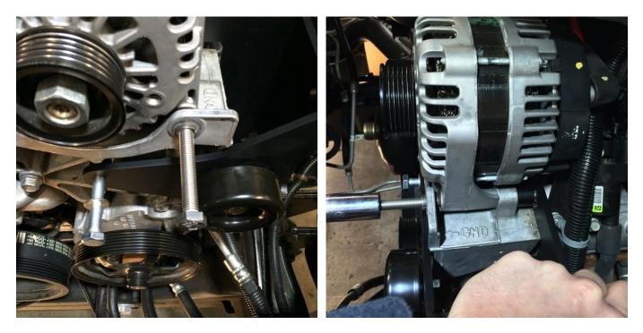
Start the threads of the partially threaded M10x130mm bolt and washer through the bracket. Install the fully threaded M10x130mm through the alternator and the bracket. It may be necessary to align the bracket with the bolt.
