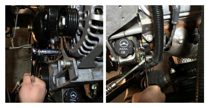
Remove the alternator bolt and accessory bracket bolts as shown. These will no longer be used. Remove the nut at the back of the power steering pump and retain. **NOTE:** Some models have a battery cable bracket attached in the 2 threaded holes shown in **Image 10**. This bracket can be angled by hand to sit behind the new compressor bracket.
