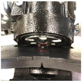
**Kits with parking brake calipers** should be checked to confirm the pad is seated flat against the piston face, with the boss of the brake pad lining up with the notch in the piston face.
