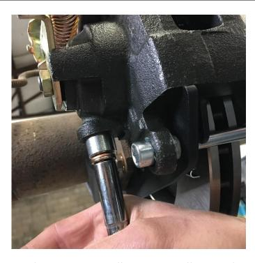
Install the banjo bolt and crush washers onto the hose as shown. If your hose has an offset, place the offset side of the fitting **away** from the caliper. Then install the hose onto the caliper as shown.
