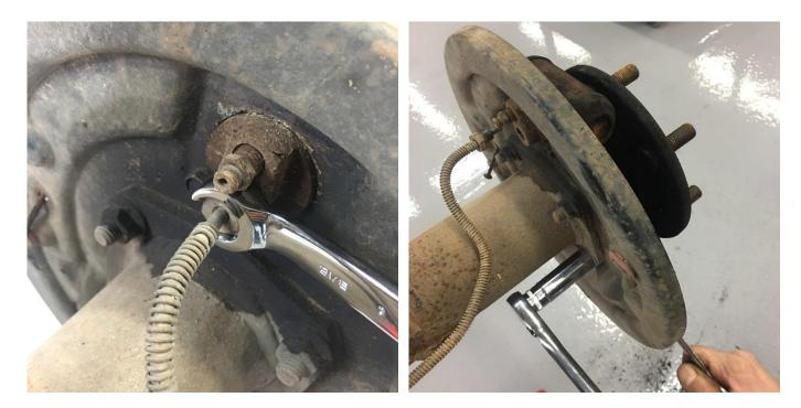
Remove the brake line from the wheel cylinder using a line wrench if possible. The 4 bolts retaining the drum backing plate to the axle can now be removed and discarded.
