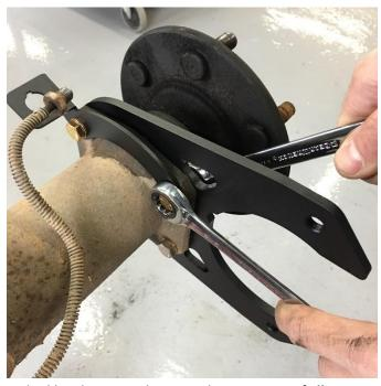
Bolt on the brackets using the supplied hardware as shown and torque to **20 ft-lbs**. Your caliper should be mounted to the **REAR** (back) of the axle.
