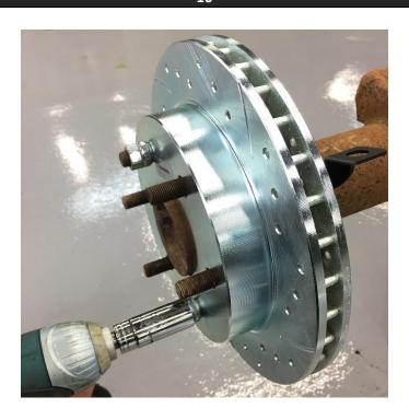
The rotor can now be installed using 2 lug nuts to temporarily secure it. In the case of drilled/slotted rotors, the direction of rotation shown is for the **passenger side**. **NOTE:** Verify that the rotors are sitting flat against the axle shaft.
